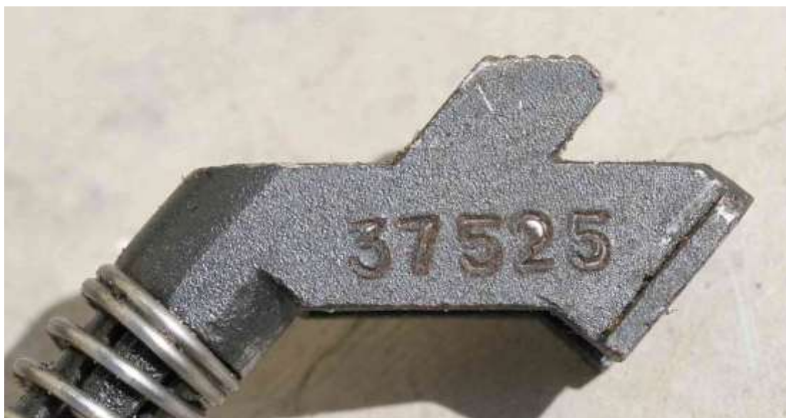
Last five digits of the serial number repeated on the recoil spring guide of the same Type 56-1 assault rifle pictured in the previous image. The marks remain intact.
