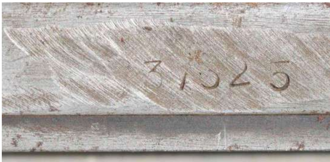
Unsuccessful attempt at grinding the last five digits of the serial number from the bolt carrier (internal component) of the same Type 56-1 assault rifle pictured in the previous image.
