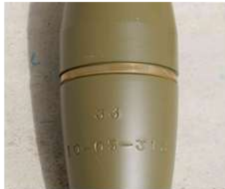
Left image: Marks designating details of the complete bomb: factory code ('313'), date code ('05'), and lot code ('9'). Right image: Marks designating details of the bomb casing (manufactured earlier in the production process): factory code ('313'), date code ('05'), and lot code ('10').
