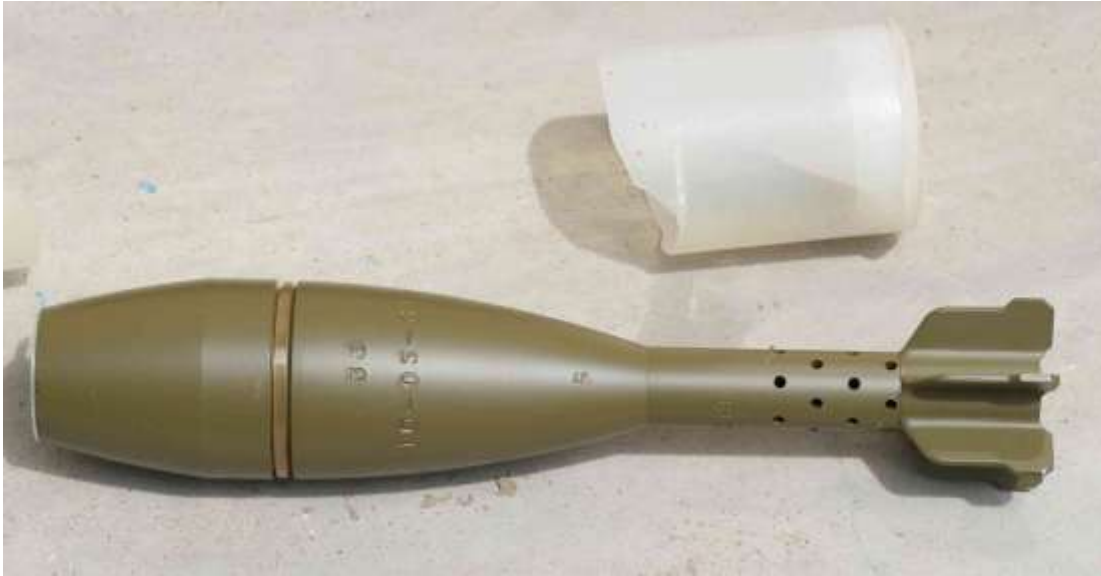
Chinese-manufactured 60 mm mortar bomb found inside a sealed tube. Subsequently removed and documented (marks documented in images below).
