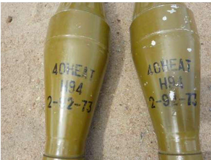
Chinese-manufactured high explosive anti-tank (HEAT) rockets for use in RPG-7-type weapons. The markings on these items indicate, from right to left: factory code ('73'), date code ('92'), and lot code ('2'). The date code '92' indicates manufacture in 1992. Rounds with the same lot number were seized from the Ethiopian Ogaden National Liberation Front (ONLF) in September 2010. A similar RPG-7 round with marks '8-91-93' was also seized from George Athor's forces in February 2011, which matched another batch of rounds that were seized from the ONLF during the same action.
