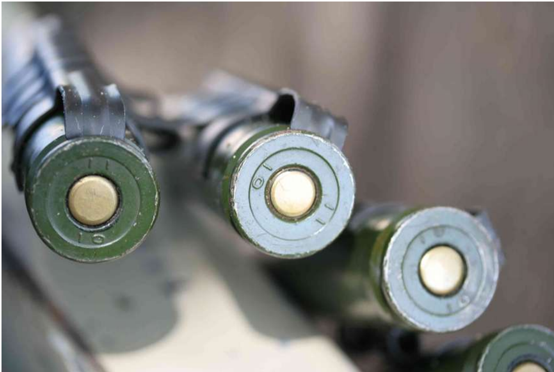
Linked, Chinese-manufactured 12.7 x 108 mm ammunition, found accompanying two vehicle mounted Type 85 heavy machine guns. The ammunition is marked with a factory code ('11') and a date code ('10'), indicating 2010 production.
