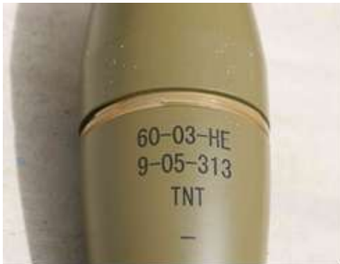
Left image: Marks designating details of the complete bomb: factory code ('313'), date code ('05'), and lot code ('9'). Right image: Marks designating details of the bomb casing (manufactured earlier in the production process): factory code ('313'), date code ('05'), and lot code ('10').
