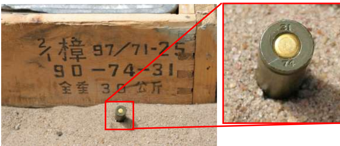
Markings on a box containing 1,500 rounds of Chinese-manufactured 7.62 x 39 mm ammunition. The marks on the box indicate, from right to left: factory code (31), date code (74), and lot (90). Cartridge headstamps (inset) feature the factory code '31' and a date code '74,' which indicates manufacture in 1974.
