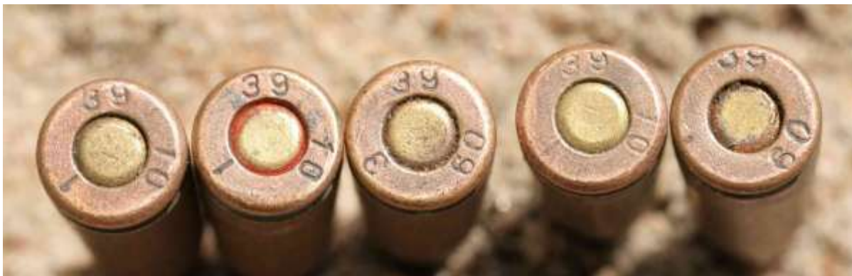
Sudanese-manufactured 7.62 x 39 mm ammunition found loose (unboxed). The ammunition headstamp features three entries: calibre ('39'), date ('10' or '09'), and what appears to be a lot or batch designator ('1' or '3'). Date marks suggest the ammunition was manufactured in 2009 and 2010. For further information, see the HSBA publication 'A Guide to Sudanese Ammunition (1954-present).' The Small Arms Survey has observed similar varieties of ammunition throughout Sudan and South Sudan.
