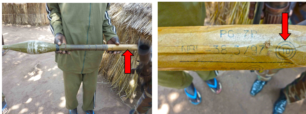
PG-7P propellant charge manufactured in Bulgaria in 1997 (left and right photos). The encircled '10' denotes Bulgarian production.
