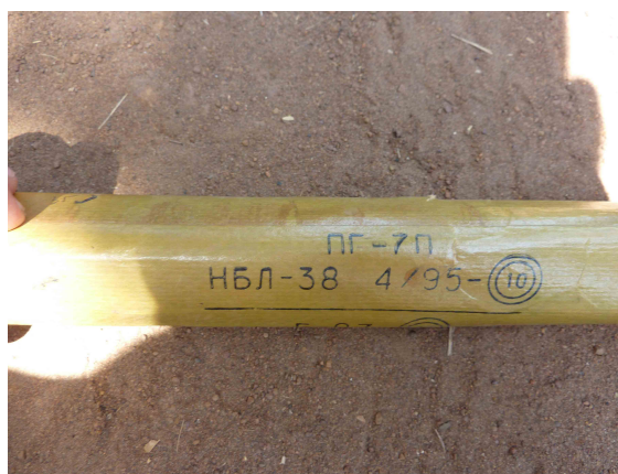
An identical PG-7P propellant charge manufactured in Bulgaria in 1995. The encircled '10' denotes Bulgarian production.
